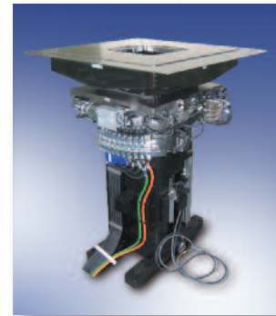
6-axis sample stage: A compact, fully integrated stage including 3 translations and 3 rotations for the positioning and orientation of loads up to 150 kg. The sphere of confusion of the 3 rotation axes is 25 \mu\text{m} . ▶
