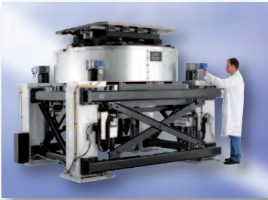
◀ Sample positioner: 2-ton sample positioner for Neutron synchrotron.
