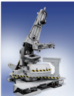
◀ X-ray diffractometers are full custom and turnkey systems used to study the structure and properties of materials. Over 30 diffractometer systems in synchrotrons all over the world serve the scientific community in a large variety of application fields.
