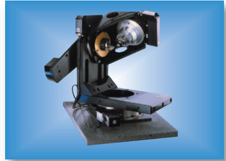
▲ Antenna and sensor positioner to measure signals in 3D for guidance and field communication systems.
